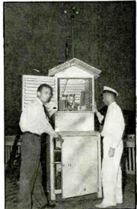
Photo—Science Service Wilbur S. Hinman, Jr., left, radio engineer of the National Bureau of Standards, and C. A. Kelly, chief aerographer of the U.S. Naval Air Station, Anacostia, D. C., watch the self-contained weather observing station observe the storm that is coming. The record untouched by human hands is sent by radio to a distant office. (See photo on cover.)
